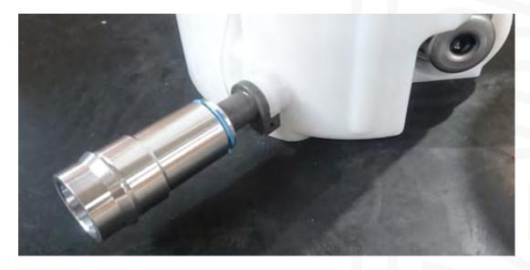
Install new fuel pump/sender module. Whilst installing, connect new crossover pipe to bottom of module onto the adaptor, orient module correctly and lock ring clockwise.
